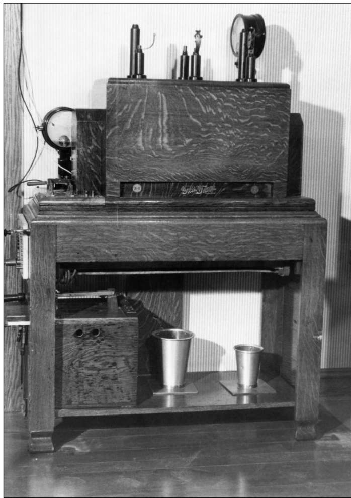
Grosse Flamme, arranged for compact museum exhibit; includes an induction coil, x-ray tube and tube stand
